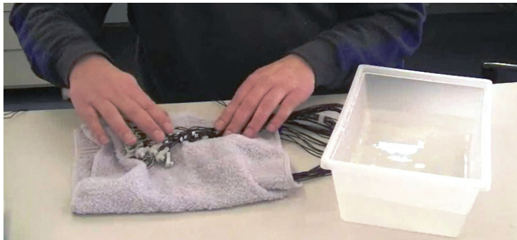
Figure 4-4. Wrap the electrodes in a towel after cleaning
