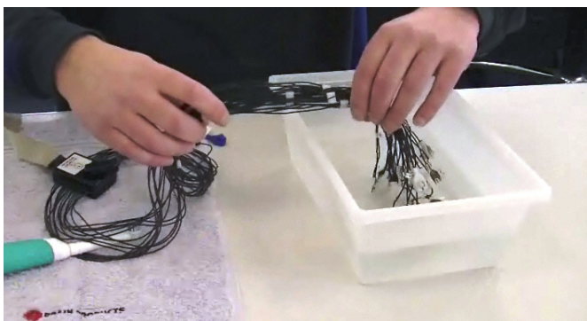
Figure 4-2. Electrodes in the water bath
